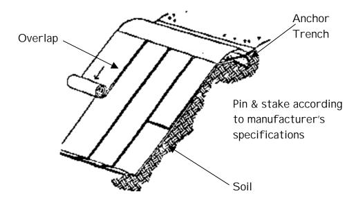
Figure 710.4 Typical RECP installation
