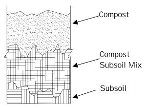
Figure 710.3 Soil Profile After Tilling to Mix Soil Layers
