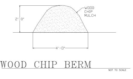
Figure 710.6 Wood chip berm detail
