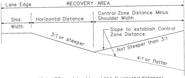
RECOVERY AREA = (shoulder width)+(horizontal distance) +(control zone distance - shoulder width)
