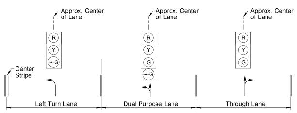
One Through Lane, a Dual Purpose (Left or Through) Lane and One Left Turn Storage Lane With Split Phasing for Protected Left Turns
