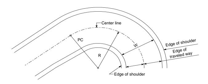
Traveled Way Width for Two-Way Two-Lane Turning Roadways Figure 640-7a
