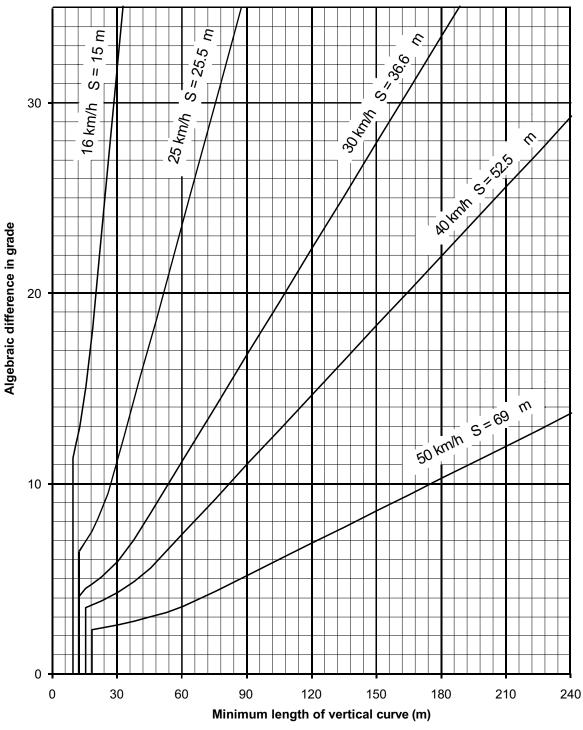
$$L = \frac{AS^{2}}{100 (\sqrt{2h_{1}} + \sqrt{2h_{2}})^{2}} \text{ when } S < L$$
