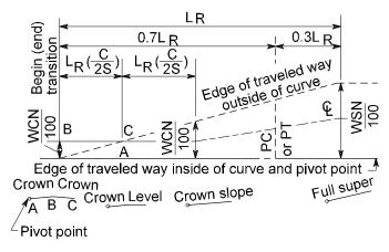
Design B<sup>2</sup> Pivot Point on Edge of Pavement Inside of Curve Crowned Section
