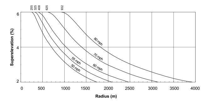
Superelevation Rates (6% max)
