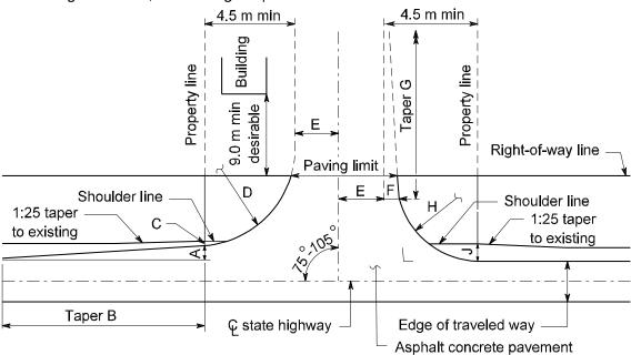
Note: Vertical curves between the shoulder slope and the approach grade not to exceed a 85 mm hump or a 50 mm depression in a 3.0 m chord.
