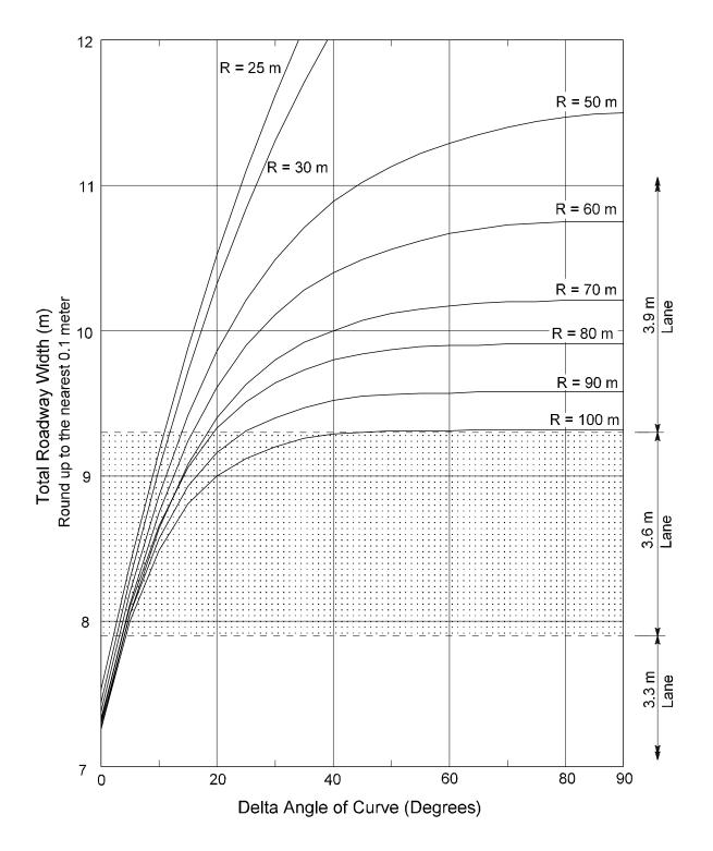
If result is less than the total roadway width from Figure 430-4 use the greater.
