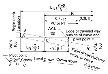
Design B<sup>1</sup> Pivot Point on Edge of Pavement Outside of Curve Crowned Section
