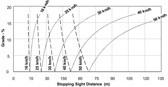
(based on 2.5 seconds reaction time)
