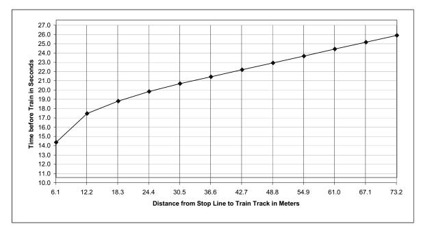
**Example:** A location where it is 18.3m from stop bar to nearest rail of a single track crossing. **Solution:** Enter table at queue length of 24.4m (18.3m + 6.1m to RR stop bar). Read 19.3 seconds.
