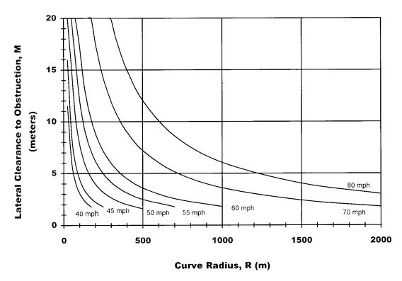
When the intersection of the lateral clearance (M) with the curve radius (R) falls below the curve for the selected design speed, corrective action must be considered.
