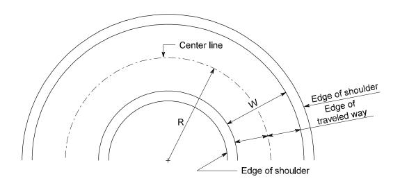
Traveled Way Width for Two-Lane One-Way Turning Roadways Figure 640-8a
