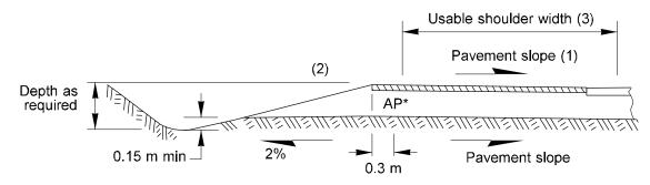
Shoulder Design on the High Side of the Roadway on Curves and Divided Roadways Shoulder Slopes with Roadway
