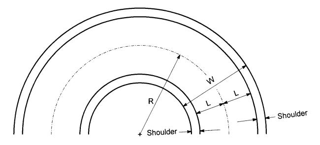
Minimum Total Roadway Widths for Two-Lane Highway Curves Modified Design Level Figure 430-5
