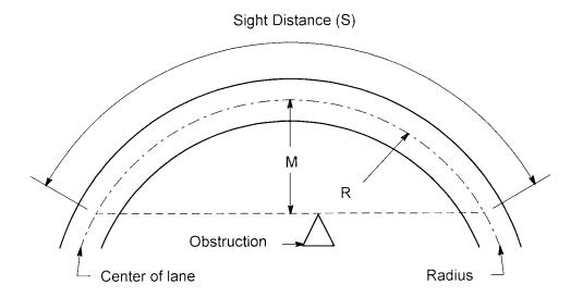
M is the distance in meters from the center line of the inside lane to the obstruction.
