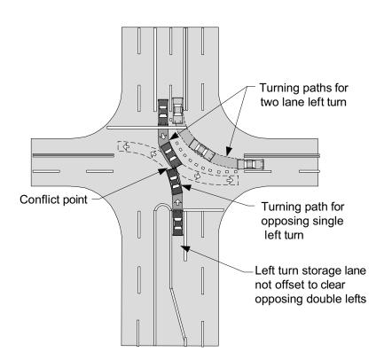
Turn Lane Configuration Preventing Concurrent Phasing Double Left Turn Channelization
