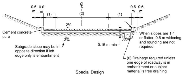
This special design section is to be used only when restrictions (high right of way costs or physical features that are difficult or costly to correct) require its consideration.
