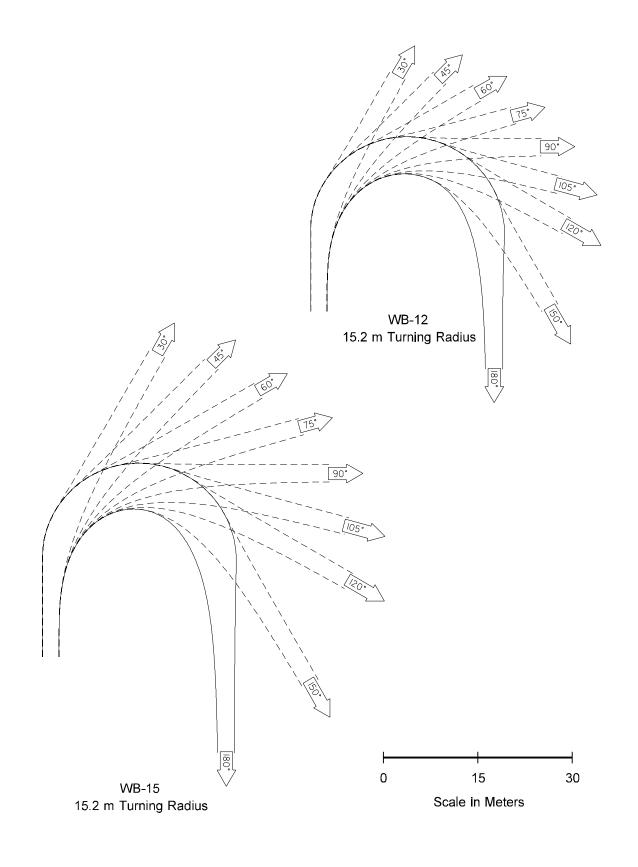
Turning Path Template Figure 910-<u>7</u>b
