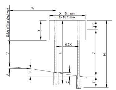
${\bf Z} = {\bf Height}$  from ground line to midheight of sign at the centerline of the longest post
