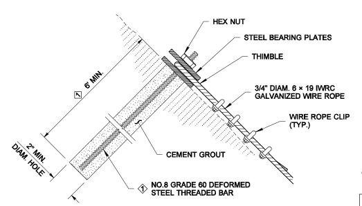
TYPE 6 **DEFORMED STEEL THREADED BAR** (FOR USE IN ROCK)
