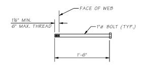
ANCHOR DETAIL ASTM A-307
