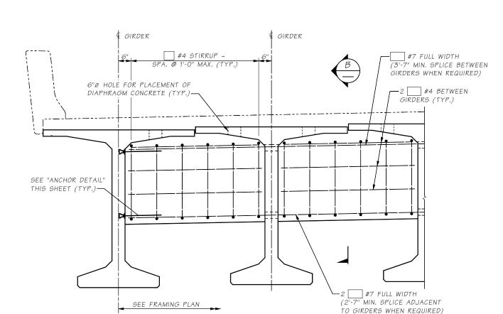
ELEVATION PARTIAL DEPTH INTERMEDIATE DIAPHRAGM
